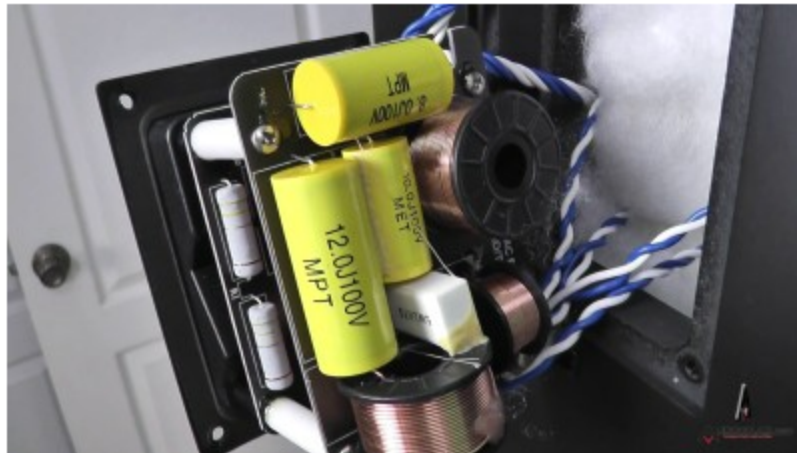
XTZ M6 Crossover and Cabinet Lined with Foam and Stuffed with Polyfill
